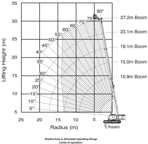
Limits of operating Kange Limits of operation: Maximum load capacity = 340 kg Maximum radius when mounted on main boom = 15.2 m Maximum occupancy = 2 persons
