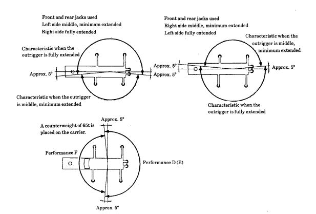
3) When the boom length and the boom fixing pin condition are other than those stated in the chart "Boom length and the boom fixing pin condition" in item 5. 2), the maximum total rated load for each boom length is limited as shown in the following table. The rated total loads below the limit value remain as they are and are the same when the boom fixing pin is used. However, when removing the boom fixing pin, the total rated loads for every boom length should be 25 tons or less.
